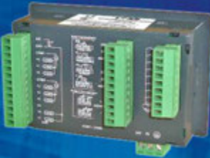
Back view for HMI with built-in Digital & Analog I/O
