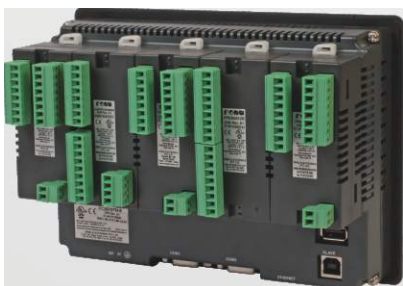
7" TFT Color LCD with Pluggable I/O Modules
